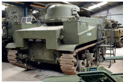
Left: The exhaust system vented in two fishtail-shaped pipes. This restored M3 Lee is at the Armourgeddon Military Museum in Leicestershire
